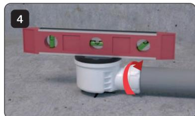
Level the waste outlet and fix it to the pipe by tightening nut and joint. Check no leakage appears.
