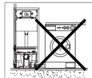
**SANITARY APPLIANCES** – The CICLON CC waste disposer is prepared to connect a single lavatory and three sanitary appliances (washbasin, bidet or shower), it does not allow connecting other electric powered appliances such as washing machines or dish washing machines, equipped with pumping devices which may interfere the correct working of the unit.
