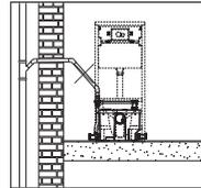
**AVOID DIAGONAL STRETCHES** – Evacuation pipes must be always installed vertically or horizontally, but never diagonally.
