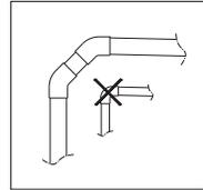
**PIPE** – For the discharge use a Ø32 mm pipe. Do not thump or make siphons with the pipe that may retain certain objects and cause obstructions. Other pipe diameters might be used (Ø28-22 mm) with the joint adapter and metal clamping supplied.
