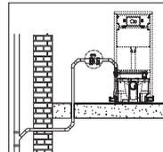
**CONNECTION TO THE FLUSH** – The connection to the flush must be carried out by means of a inclined branch. If the connection to the flush is at a lower level regarding the waste disposer base, a A-69 Jimten-type venting valve must be set at the highest point in the installation to prevent the waste disposer from being emptied.
