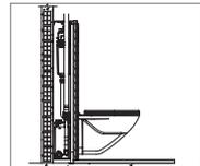
**VENTILATION** – The waste disposer unit must be placed right behind the lavatory, it should never be installed in wall-embedded installations, behind walls, etc, which avoid the correct ventilation of motor, which incorporates a self ventilating mechanism.
