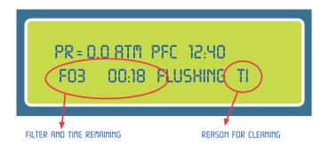
In this example, filter 3 is being cleaned, with 18 seconds remaining before cleaning the next filter. It is also indicating that this cleaning process has been started by time counter (TI).
