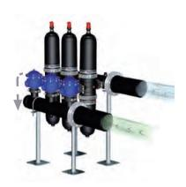
Our range has different filtration degree color-coded discs depending on the total suspended solids of raw water to be filtered and our automatic filtration stations are designed to match flow requirements of the installation. The cartridge spine has an internal piston spring for compressing or releasing the discs during the filtration and backwash cycles.
