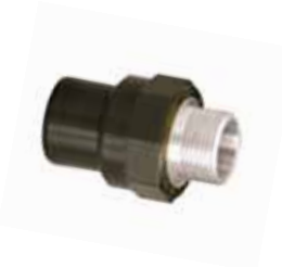
HEAS Terminal rosca macho CPVC-Acero Inox. AISI316 H/M encolar - M roscar ac. inox.
